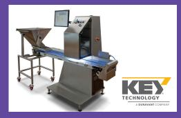
Automation Series AS40 Conveyors are an integral part of Key Technology's VeriSym SE, a visual inspection and reject system for pharmaceutical soft gels.
