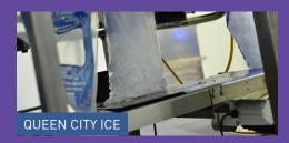
As an SQF-Certified facility, Queen City Ice was drawn to HydroClean Series conveyors due to their easy-to-clean design that requires no tools for disassembly. The conveyors must be able to operate in the cold, wet environment of an ice plant and withstand being washed down every day.
