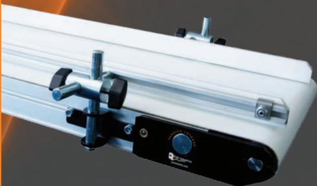
Adjustable side rails offer the ultimate in flexibility. Available guide heights are 1" (shown), 2", and 3". Standard guides may be adjusted approximately 3" vertically and horizontally. These guides are available with optional thumb screws (shown) for tool-less adjustments.
