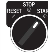
**4** Start conveyor by turning control switch to Start (↕)
