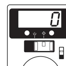
**3** If controller displays "0" the alarm has been cleared
