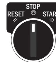
**1** Stop conveyor by turning control switch to Stop (⊖)
