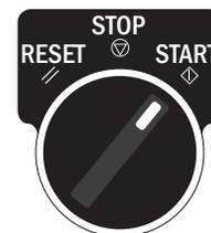
EN **1** Start conveyor by turning control switch to Start (↕)
