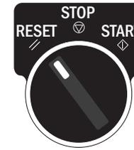
**2** Turn control switch to Reset (↗) hold for one second
