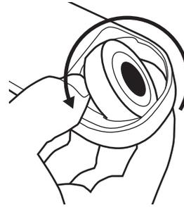
**7** Rotate new bearing into housing
