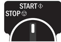
**4** Replace plastic cover on controller box and turn Start/Stop switch to start (◊)
