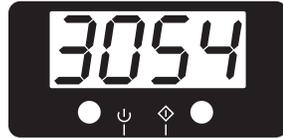
**2** Rotate dial on controller until desired speed is displayed
