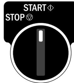
EN **3** Start conveyor by turning Start/Stop switch to Start (◊)
