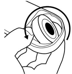
EN **8** Rotate new bearing into housing
