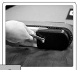
Remove the black plastic covers from the tail pulley assembly. Use a 7/16" wrench to remove nuts and slide black cover off. Repeat for both sides.
