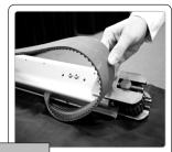
Remove the belt by sliding it over the tail pulley and bracket. Next slide the belt out of the flange on the underside of the frame and off the conveyor. Note: Use extreme caution when removing the belt, the tail pulley assembly can slide out of the brackets.
