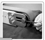
Using a 3/16" Allen Wrench, rotate the two 3/8-24 Socket Head Set Screws counter-clockwise to move the tail pulley toward the conveyor frame.
