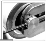
Rotate the 3/8-24 Socket Head Set Screws until the lines meet up on the tail pulley and bracket. Do this for both sides to apply the proper tension.
