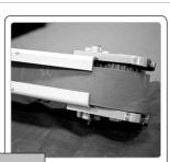
Start by sliding the belt over the drive pulley of conveyor, then over the tail pulley. Next slide the belt into the C-Flange on the underside of the frame. Do this down the entire conveyor length.
