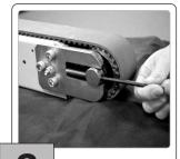
Using a 3/16" Allen Wrench, rotate the two 3/8-24 Socket Head Set Screws clockwise to move the tail pulley back away from the conveyor frame. If tail assembly bracket was removed earlier (for wider conveyors), reinstall the bracket, jam nuts and stud first.
