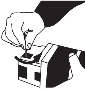
**9** Back set screw out of coupler half allowing space for key in key way.
