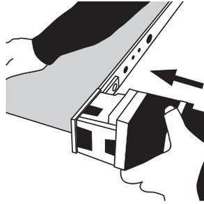
**10** Slide speed reducer assembly onto conveyor's shaft and hold in place.
