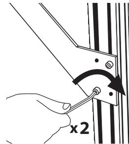
**7** Tighten socket head cap screws and repeat process on other side of conveyor.
