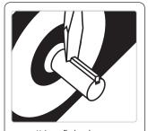
Using a flathead screwdriver, lightly strike just behind the key to ensure key does not slide.
