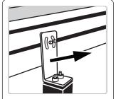
Remove mounts on one side of conveyor using steps outlined in Mount Install section of this manual. (Only remove one mount at a time to keep conveyor stable. Replace each mount as belt is removed)
