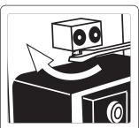
Loosen jacking screw, moving speed reducer or motor away from conveyor and apply tension to drive belt.
