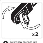
Rotate new bearings into bearing housings.
