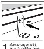
rection foot will face, insert two cap screws through mount and into t-slot.
