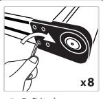
Tighten four screws on 10 lighten four screws on each side of conveyor to secure drive pulley assembly.
