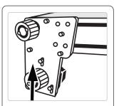
Slide bottom sprocket up to reduce distance between sprockets.
