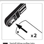
Install drive pulley into bearings with drive shaft facing proper direction.
