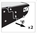
Remove twist nut on both Remove twist..... sides of tail assembly.
