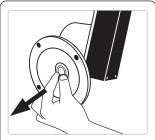
Remove plug from speed reducer.
