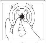
Rotate quill pin on speed reducer so that keyway is in 12 o'clock position.
