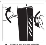
Loosen but do not remove safety bolt.
