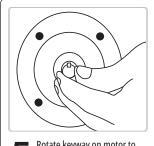
Rotate keyway on motor to 12 o'clock position.
