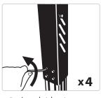
Looen but do not remove Looen but do not remove four cap screws holding bracket to frame legs.
