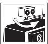
Tighten jacking screw allowing movement of speed reducer or motor.
