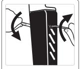
Tighten safety bolt. If height adjustment moved added slots above top of stand legs, bolt may be removed and replaced at lowest available slot before tightening, but is not required.
