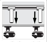
Align adjustment rods with cross blocks on mounts, and tighten into place along guide.
