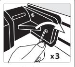
5 Tighten three cap screws of secure mounting package Tighten three cap screws to to conveyor.
