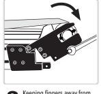
Keeping fingers away from 6 Reeping inigers a..., all pinch points, rotate tail pulley back down into engaged position.
