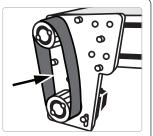
Install belt over both sprockets and check for alignment.
