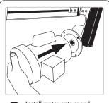
Install motor onto speed reducer.
