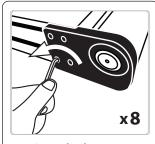
Loosen, but do not remove, four mounting screws on each side of drive assembly.
