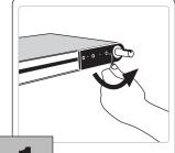
Remove and discard three cap head screws from drive side bearing block. (Leave bearing block in place)
