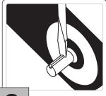
Using a flathead screwdriver, lightly strike just behind the key. This will stop it from sliding.
