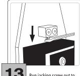
Run jacking screw out to create tension on belt. (Approximately 6lbs of force to deflect one span of belt .09")
