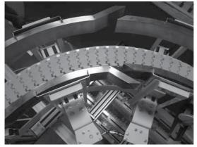
Automated side guide installed at bend section
