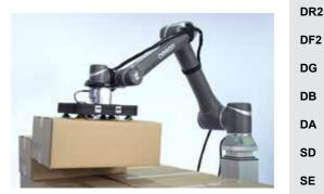
Cobot Palletizing using Omron Cobot
