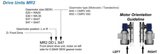
Example. Code for Basic unit; MR2 DD R S47 => Front drive unit, motor on right side for SEW SA47 gearmotor.
