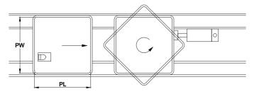
This module is used when a pallet needs to be located and rotated to desired orientation according to the machine needs
