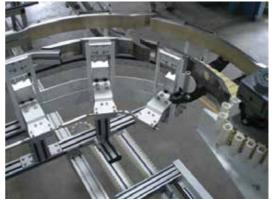
Automated side guide installed at bend section
