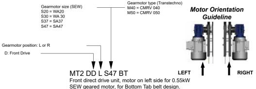
Example. Code for Basic unit; MT2 DD R S47 BT => Front drive unit for bottom tab chain, motor on right side for SEW SA47 gearmotor.
