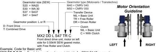
MX2 DD R S47 => Front drive unit, motor on right side for SEW SA47 gearmotor.
