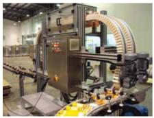
Gripper Conveyor System Intergrated with Can Cleaner to Remove Dust Particles from the Can
