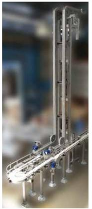
S-Flow Gripper Conveyor to Elevate Carton Boxes
