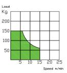
The diagram shows the maximum permissible weight of a group of pallets (product weight+pallet weight) comparison with the conveyor speed.
