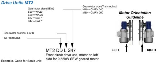
MT2 DD R S47 => Front drive unit, motor on right side for SEW SA47 gearmotor.
