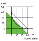
The diagram shows the maximum permissible weight of a group of pallets (product weight+pallet weight) comparison with the conveyor speed.
