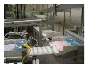
Side Transfer Unit for Optical Trays
