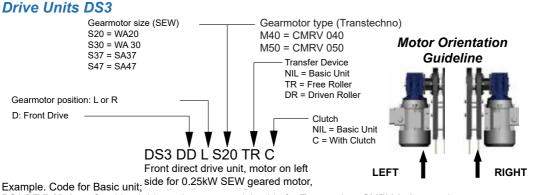
DS3 DT R M50 => Combined drive unit, motor on right side for Transtechno CMRV 050 geared motor.
