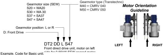
**DT2 DD R S47** => Front drive unit, motor on right side for SEW SA47 gearmotor.
