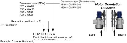
DR2 DD R S47 => Front drive unit, motor on right side for SEW SA47 gearmotor.
