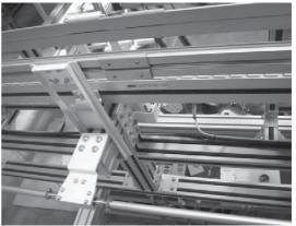
Automated side guide installed at straight section
