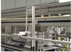
Automated side guide installed at straight section
