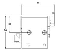
Pallet stop, damped, 0–35 kg Pressure range : Treated compressed air: 4–8 bar Air connection : 6 mm outside diameter tubing
