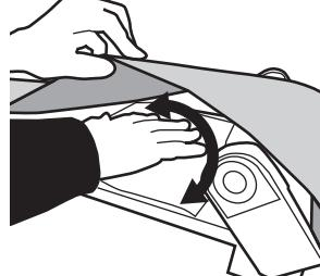
**11** Wipe the entire length of the frame underneath the conveyor belt.
