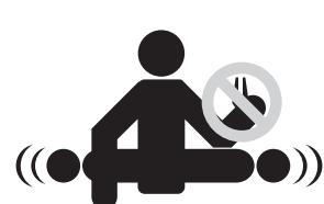
Servicing equipment that is moving or energized can cause severe injury. LOCK OUT POWER prior to performing maintenance.
