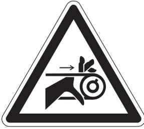
EN When used improperly, the conveyor rollers can pinch or maim.
