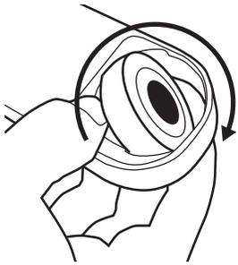
EN **5** Rotate old bearing out of housing
