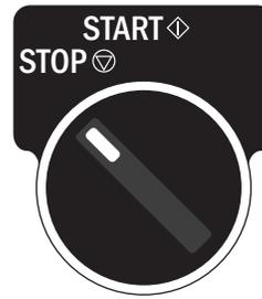
EN **1** Stop conveyor by switching Start/Stop switch to Stop (○)
