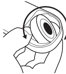
**7** Rotate new bearing into housing
