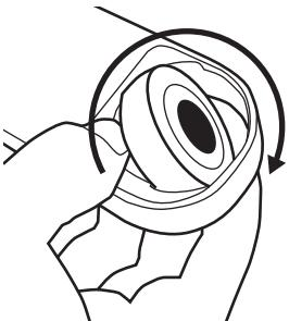
**6** Rotate old bearing out of housing
