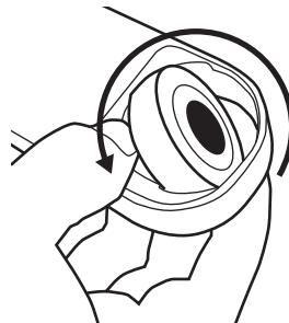
**8** Rotate new bearing into housing
