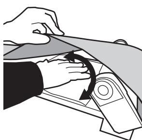
**12** Wipe entire length of frame underneath conveyor belt
