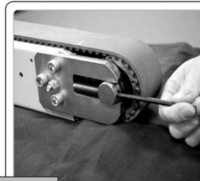
**2** Using a 3/16" Allen Wrench, rotate the two 3/8-24 Socket Head Set Screws clockwise to move the tail pulley back away from the conveyor frame. If tail assembly bracket was removed earlier (for wider conveyors), reinstall the bracket, jam nuts and stud first.
