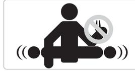
Servicing equipment that is moving or energized can cause severe injury. **LOCK OUT POWER** prior to performing maintenance.
