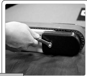
**1** Remove the black plastic covers from the tail pulley assembly. Use a 7/16" wrench to remove nuts and slide black cover off. Repeat for both sides.
