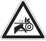
When used improperly, the conveyor rollers can pinch or maim
