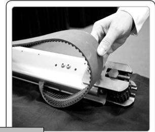
**4** Remove the belt by sliding it over the tail pulley and bracket. Next slide the belt out of the flange on the underside of the frame and off the conveyor.
